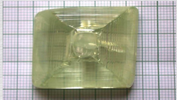
KYb 0.9 Tm 0.1 (WO 4 ) 2 single crystal Potassium yttrium tungstate doped with 10 atomic % thulium - laser crystal.
