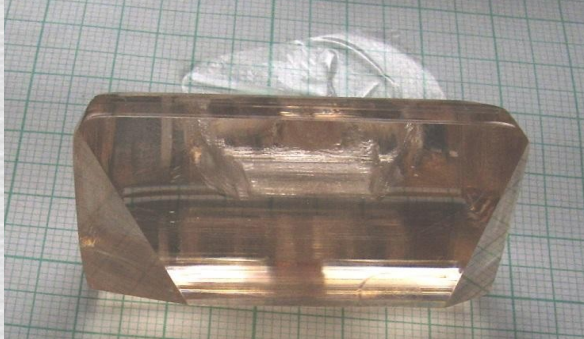
KTiOPO 4 single crystal Potassium titanyl phosphate - nonlinear optical crystal.
